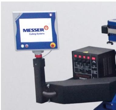
The modern cnc control Global Control and the plasma interface are mounted where the operator can easily see and adjust them.
